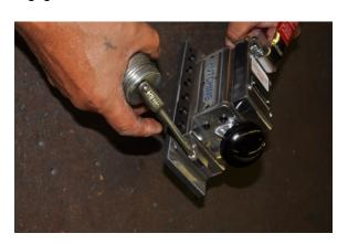
Step # 4 With pad removed, oil the right and left runner assemblies. Again be generous with the lubricant.
