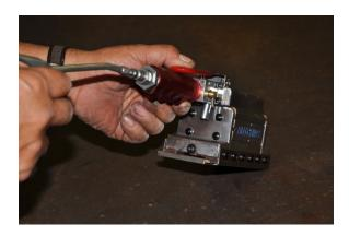
Step # 3 Squirt a generous amount of tool oil into both ends of the tool where the drive shoe engages the runner assemblies.
